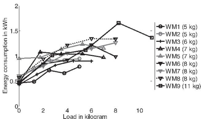
**Figure 4** Energy consumption in kWh of nine washing machines in dependence of the load size. Washing temperature is 60 °C and the detergent dosage is 100% of the nominal dosage. Lines are for visualization purposes only
