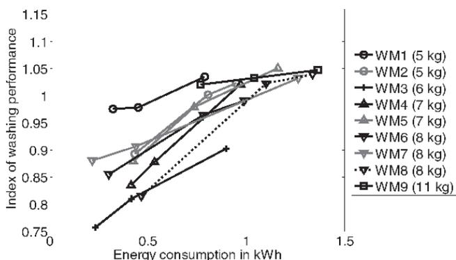
Figure 6 Index of washing performance in dependence of the washing temperatures and the respective energy consumption. From left to right the energy values indicate the washing machines' energy consumption for 30, 40 and 60 °C programs; Lines are for visualization only
