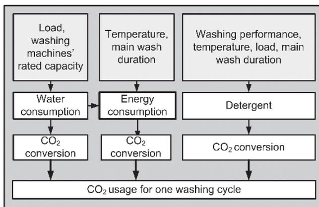
Figure 8 Schematic of a construction of a virtual washing machine and the based on the data measured during the washing machine tests
