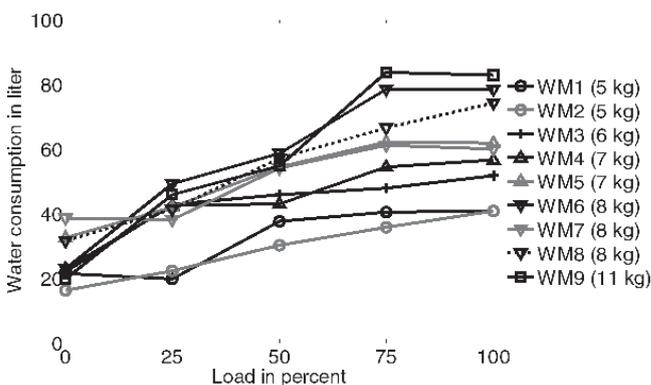
Figure 2 Water consumption of nine washing machines in dependence of the load size. Washing temperature is 60 °C and the detergent dosage is 100% of the nominal dosage. Lines are for visualization purposes only
