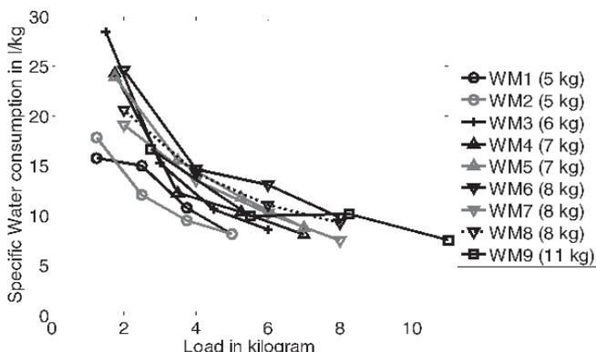
**Figure 3** Specific water consumption of nine washing machines in dependence of the load size. Washing temperature is 60 °C and the detergent dosage is 100% of the nominal dosage. Lines are for visualization purposes only
