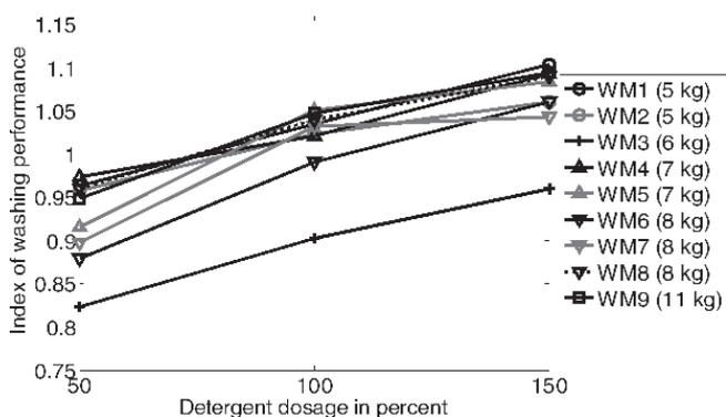
Figure 7 Index of washing performance in dependence of the detergent dosage. Washing temperature is 60 °C. Lines are for visualization only
