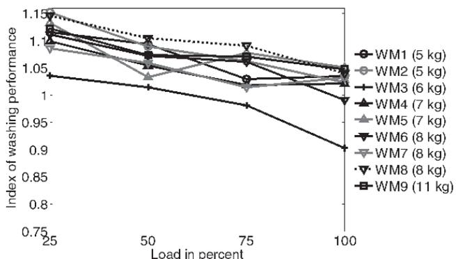
Figure 5 Index of washing performance in dependence of the load size. Washing temperature is 60 °C and the detergent dosage is 100% of the nominal dosage. Lines are for visualization purposes only
