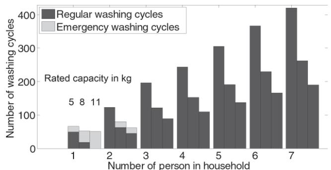
Figure 6 Yearly simulation of usage of three washing machines with a rated capacity of 5 kg, 8 kg and 11 kg. Comparison of the number of washing cycles in dependence of the household size, washing machines rated capacity and the household behavior regarding the maximal laundry waiting time. It is assumed that household waits for two weeks and washes the laundry in the third week (MLWT = 2)
