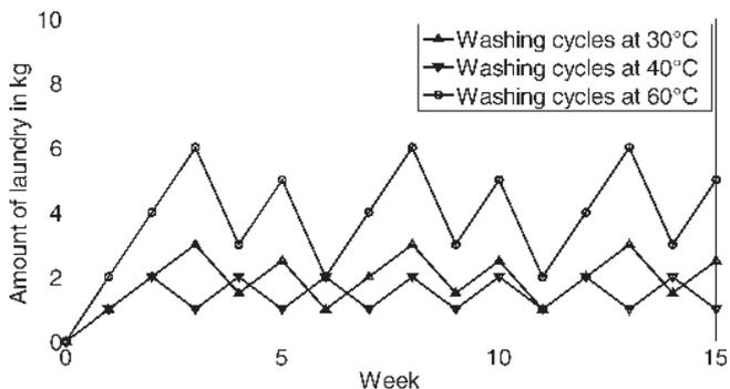
Figure 2 Example of simulation of a usage of a 5 kg washing machine for 15 weeks: comparison of three laundry stocks (30 °C, 40 °C and 60 °C laundry stock)
