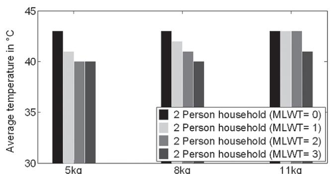
Figure 7 Comparison of average washing temperatures in dependence of the maximal laundry waiting time on an example of a 2-person household
