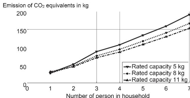
Figure 4 Yearly simulation of usage of three washing machines with a rated capacity of 5 kg, 8 kg and 11 kg. Comparison of the CO<sub>2</sub> equivalent emission in dependence of the household size, washing machines rated capacity and the household behavior regarding the maximal laundry waiting time. It is assumed that household waits for two weeks and washes the laundry in the third week (MLWT = 2)
