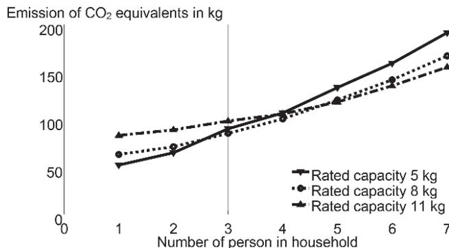
Figure 3 Yearly simulation of usage of three washing machines with a rated capacity of 5 kg, 8 kg and 11 kg. Comparison of the CO<sub>2</sub> equivalent emission in dependence of the household size, washing machines rated capacity and the household behavior regarding the maximal laundry waiting time. It is assumed that household does not wait and washes the laundry in the same week (MLWT = 0)
