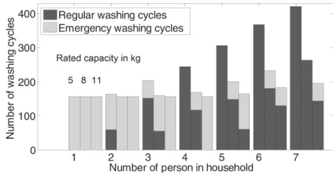
Figure 5 Yearly simulation of usage of three washing machines with a rated capacity of 5 kg, 8 kg and 11 kg. Comparison of the number of washing cycles done in dependence of the household size, washing machines rated capacity and the household behavior regarding the maximal laundry waiting time. It is assumed that household does not wait and washes the laundry in the same week (MLWT = 0)
