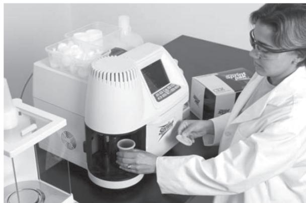
cups and filters, which contain the sample completely. At the end of a test, the non-toxic sample waste, the disposable filter and cup are discarded.
